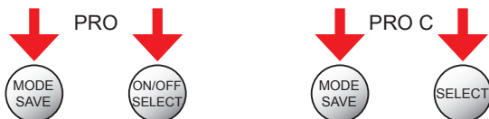
figure 15 For a manual initialization, press and hold down both buttons of the lubricator simultaneously.
